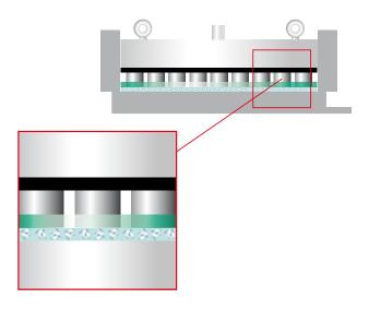
Lapping process with vehicle and loose abrasive.  $(\mathrm{SiC,\,AI_2O_3,\,B_4C})$
