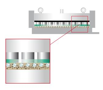
Polishing process with diamond impregnated pad. (natural or synthetic diamond)
