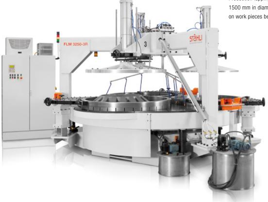
Production lapping machine for parts up to 1500 mm in diameter. Programmable force on work pieces between 0-750 daN.
