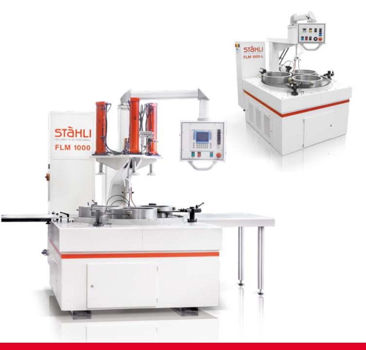
Lapping or polishing with free-rolling particles or flat honing with fixed or super abrasive wheels – the machines of our FLM 750 – 1500 range are real all-rounders. Their employment in both large and small manufacturing shops is multipurpose and includes single piece machining as well as performance oriented series production. Their technological advantages are well
